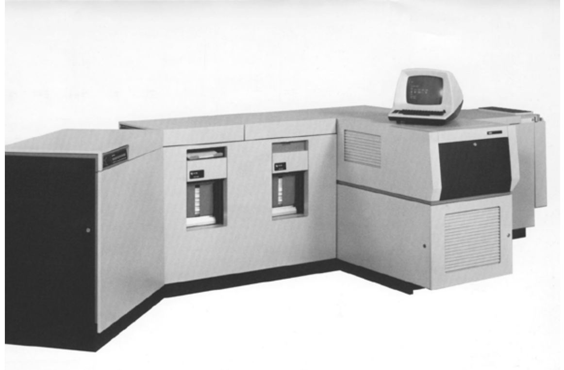
The 9700 laser printer, Xerox's first commercial laser printer, introduced in 1977, weighed more than a ton and was priced at $295,000.
